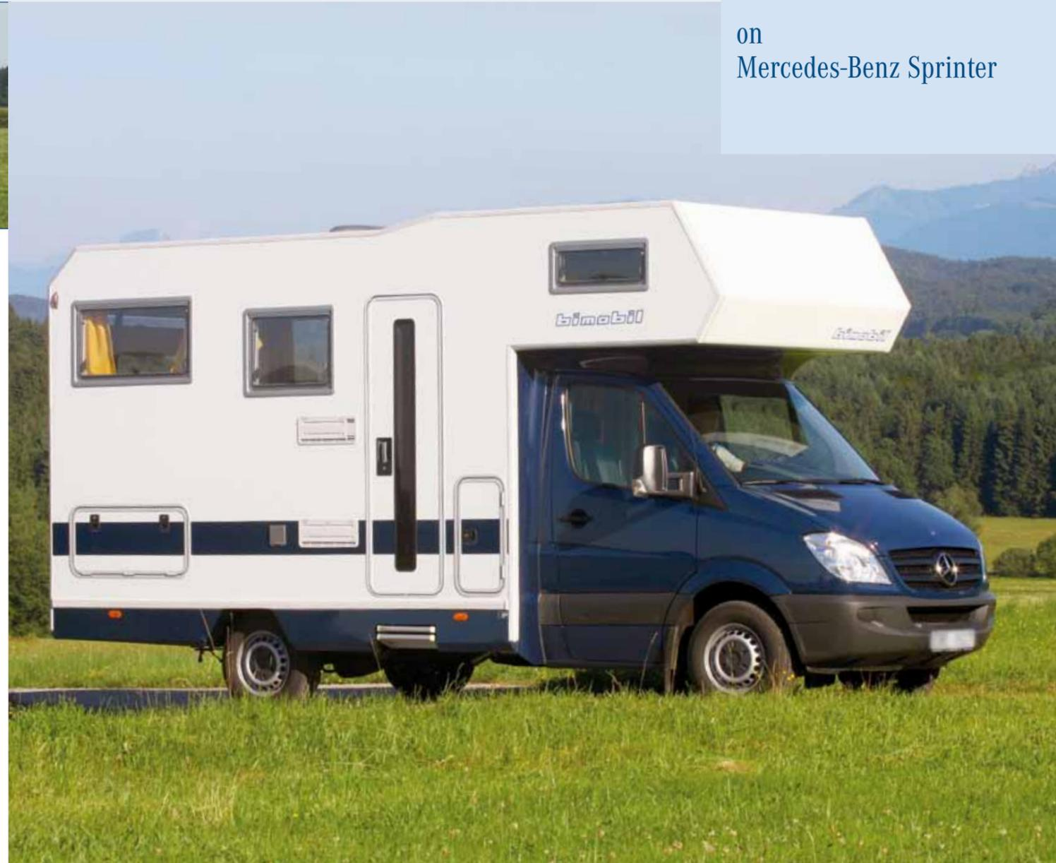
Our LB365 cabin on MB Sprinter is available for single and double-cab versions. In both cases, the vehicle can be equipped with our quick-mounting system, which enables quick and easy removal and mounting. Flat-beds or cargo compartments can be alternated with cabin for a truly dual purpose vehicle.
